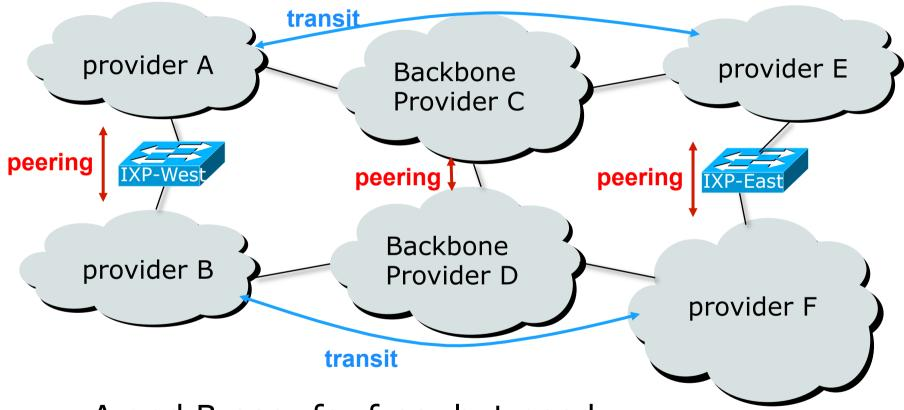
A and B peer for free, but need transit arrangements with C and D to get packets to/from E and F
